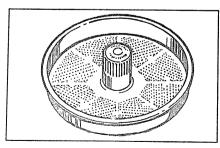
The Filter-Flo pan is the lint filter. Position the Filter-Flo pan on the agitator after loading clothes into the washer. Lint is easily seen and removed after the wash is finished.
